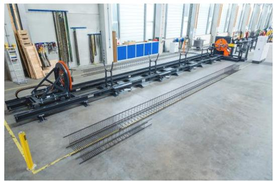
The production performance of the RSM-045 is impressive – up to 750 metres are possible per shift, depending on the cage properties. The simple handling and programming take place using a clearly arranged touch panel. The reinforcement cage and welding data can be saved very simply via the cage program, which makes things noticeably easier in day-to-day production.
