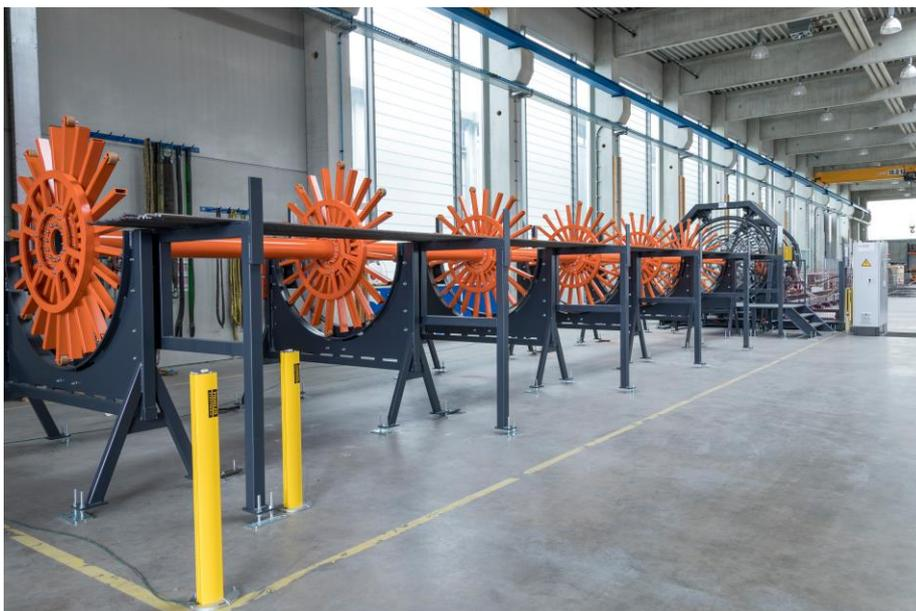
The winding wire diameter is 6-12 mm and is also available in the dimensions 6-16 mm (option); the spacing of the winding wire is located at 20-250 mm. The wire routing of the winding wire is carried out by the coil via wire guide stand and the guide rollers through the wire guide to the welding roll. A hydraulic cage support during production and cage removal is part of the stable production process.
